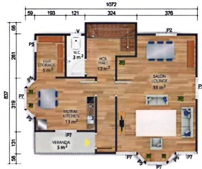
Zemin Kat Planı / Ground Floor Plan 73 m 2 + 5 m 2 = 78 m 2
